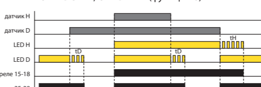
PUMP DOWN, OFF DELAY (функция 6)
